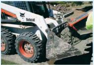
Hire a bobcat to move waste or transfer concrete from truck to trench.
